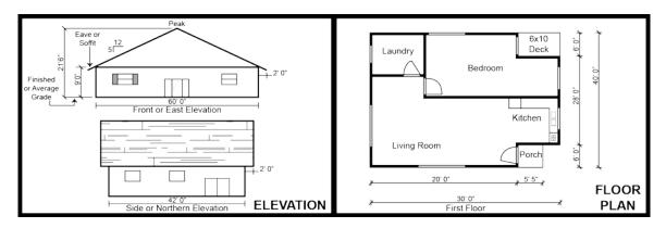
Building elevation drawings are exterior views of the building, sometimes identified as front, rear, left or right or North, South, East or West. Elevation drawings must be:
